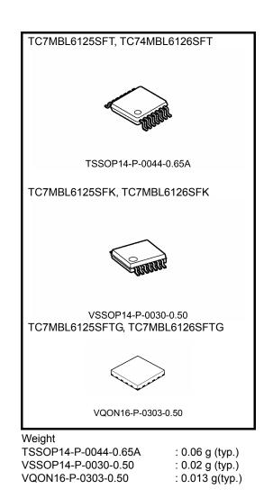
Note: When mounting VQON package, the type of recommended flux is RA or RMA.
