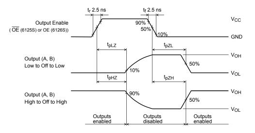
Figure 2  $t_{pLZ}, t_{pHZ}, t_{pZL}, t_{pZH}$
